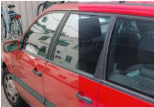
Split screen example of different images/artefacts due to polarisation
