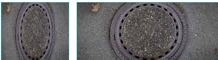
Squeezed anamorphic image as projected on sensor and de-squeezed
