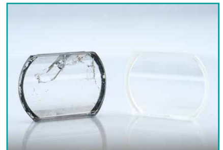
Broken cylindrical element and new replacement glass
