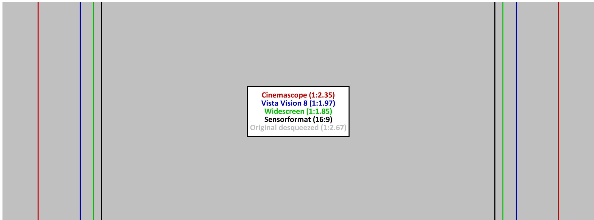
Illustration 11: Sensors with Aspect Ratio: 16:9 and Anamorphic Lens (1.5x)
