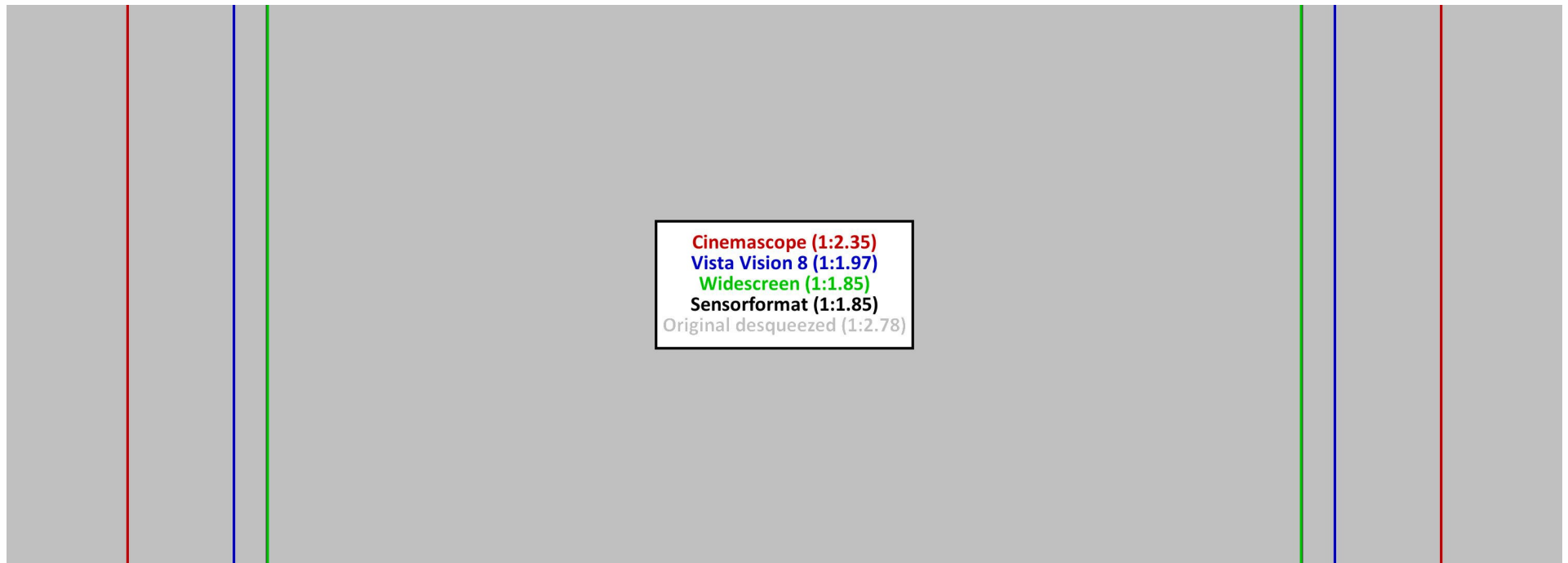
Illustration 12: Sensors with Aspect Ratio: 1:1.85 and Anamorphic Lens (1.5x)
