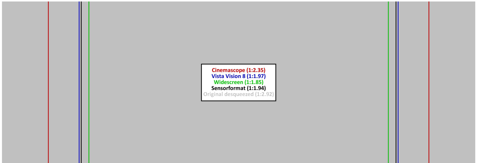
Illustrative 14: Sensors with Aspect Ratio: 1:1.94 and Anamorphic Lens (1.5x)
