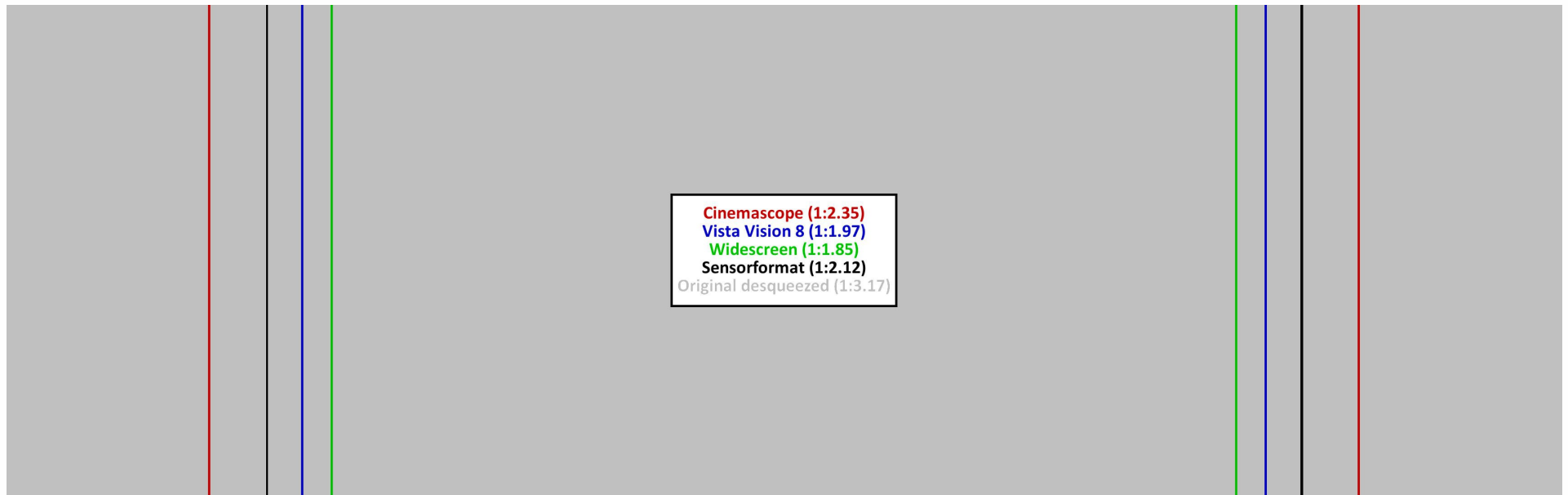
Illustration 15: Sensors with Aspect Ratio: 1:2.12 and Anamorphic Lens (1.5x)
