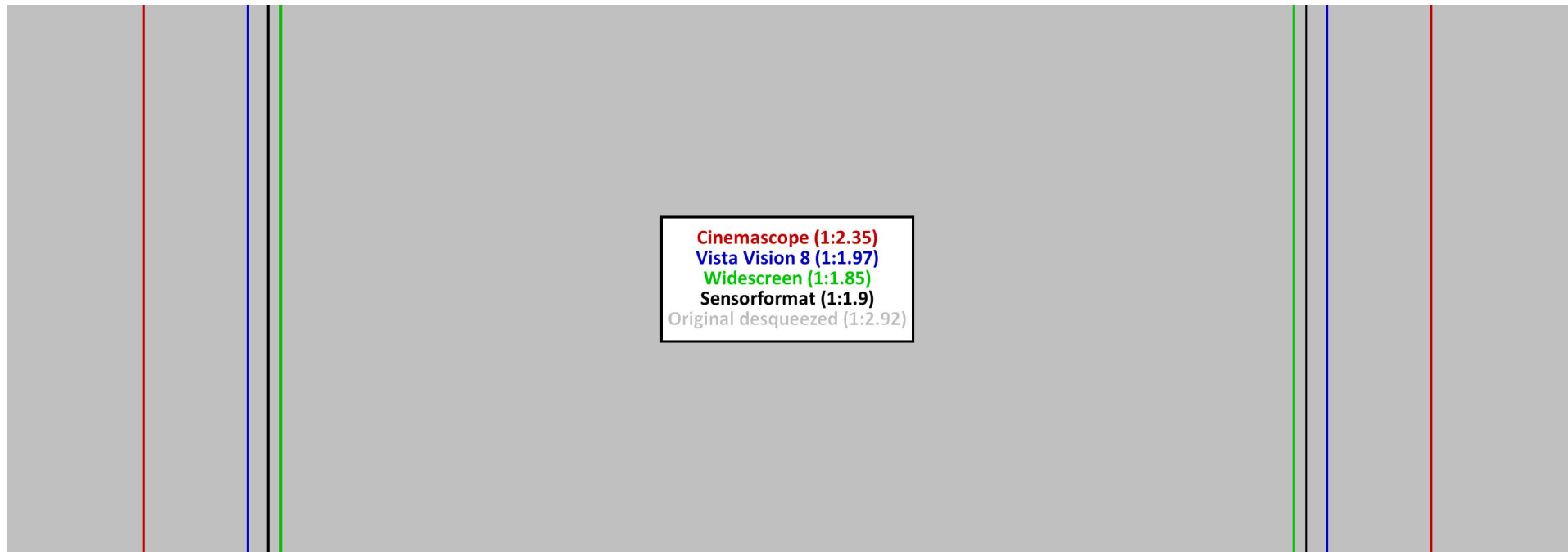
Illustration 13: Sensors with Aspect Ratio: 1:1.90 and Anamorphic Lens (1.5x)
